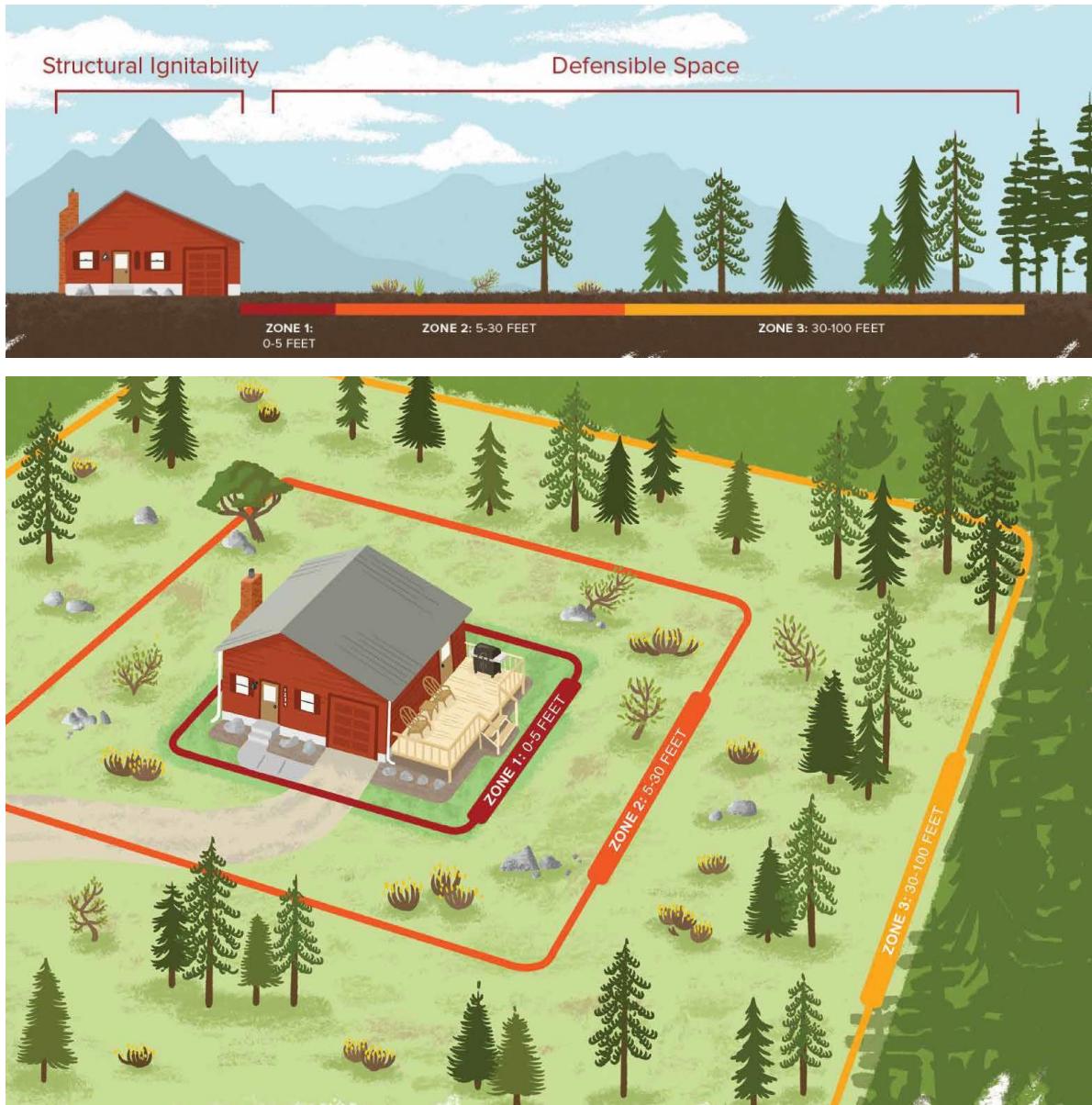
Figure 3.a.1. Home ignition zones recommended by the Kansas Forest Service. Using ignition-resistant building materials and removing burnable fuel around primary structures, outbuilding such as sheds, and campers / RVs is crucial for increasing your home's chance of surviving a wildfire and creating safe conditions for wildland firefighters.
