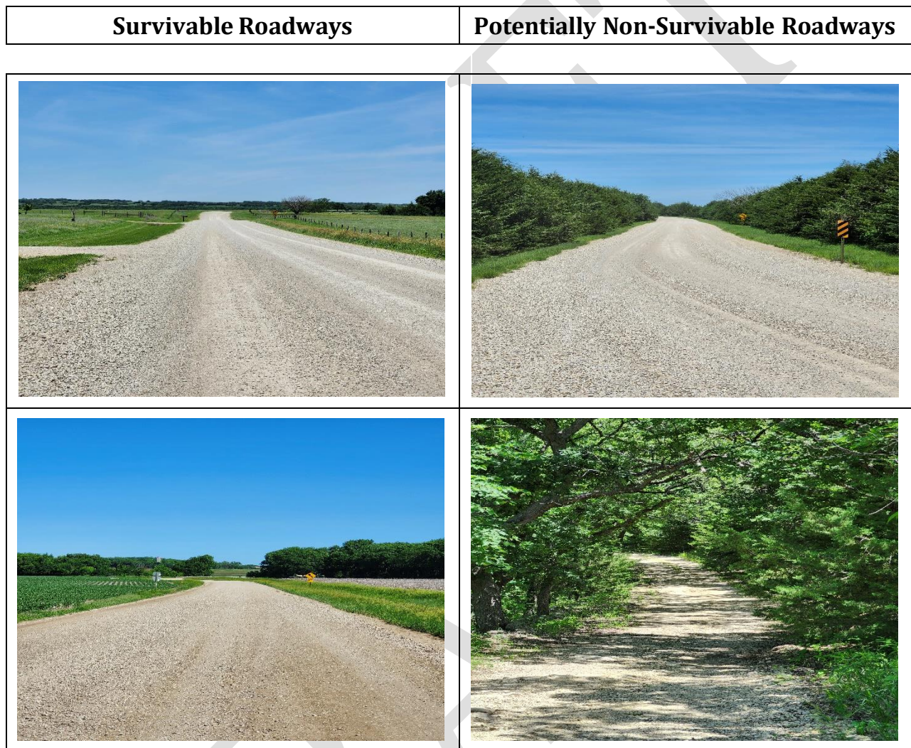
Figure 3.c.1. Some roads in Riley County have been well mitigated by removing tall trees and saplings, removing limbs on the remaining trees, and keeping grass mowed (left images). Other roads could experience potentially non-survivable conditions because they are lined by thick forests that have an abundance of ladder fuels (right images).
